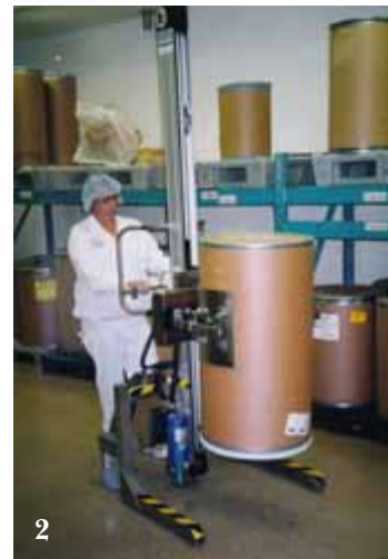
2. PRO200 with EasySqueeze unit, stainless steel.
