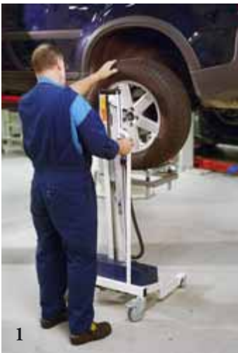
1. Choose a special tool with rolls on springs to aid in the heavy task of removing wheels.
