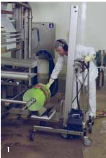
1. The PRO120 with V-block and rotating plate.
